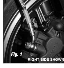
6. Bleed the system and check for leaks while applying pressure.
